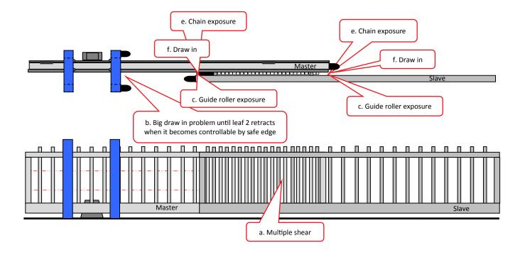
Guide roller exposure can lead to finger traps as with conventional sliding gates but is exemplified because the guide channel and rollers between master and slave leaf are more exposed and move with the leaves. The solution could be local guard or enclosure of channel, see drawing below.
