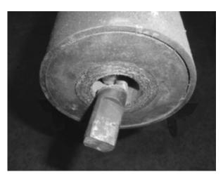
The most frequent cause of failure, injury and numerous deaths have involved some problem with the safety and security of the headgear of the door. It is for this reason that access to the headgear is crucial for maintenance. If the headgear of a door cannot be accessed, it cannot be maintained in a safe condition. The legal responsibilities of neither the owner/manager nor the maintainer can be satisfied.
