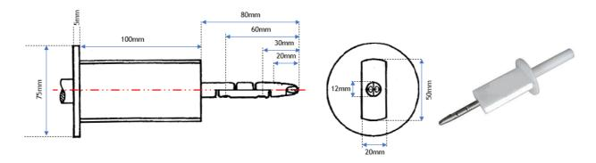
The end of the test piece tapers at  $74^{\circ}$  for 10mm and then further to  $37^{\circ}$  for the last 10mm.
